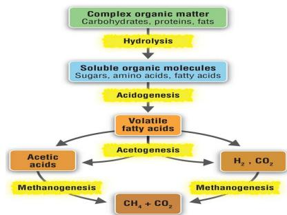
Fig.1. Different steps of anaerobic digestion process
